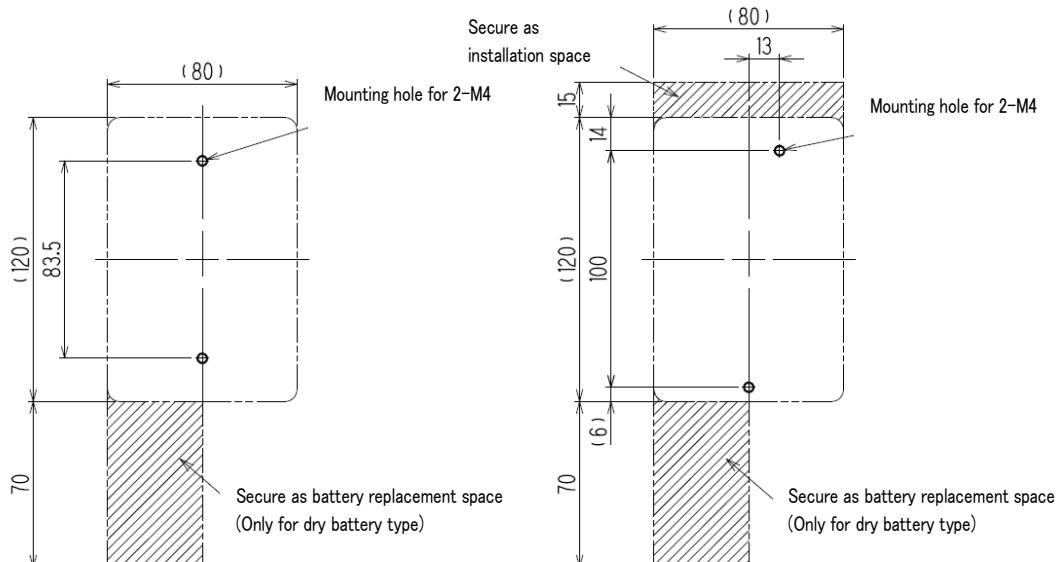
Installation dimension drawing (Installation board not used)
